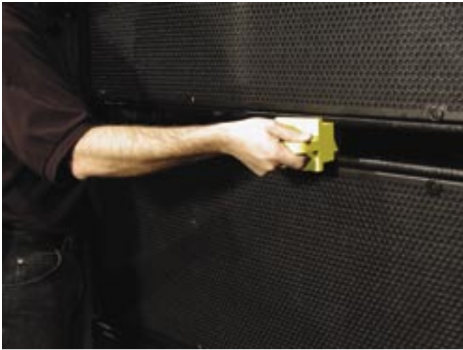
Figure 21. Adjusting angle using the alignment block
